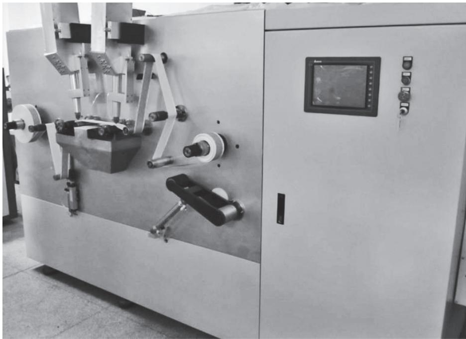
图8 “集成图形”卷烟接装纸激光打孔设备
